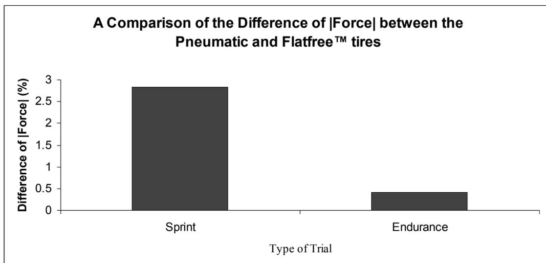
Figure 2. The absolute difference of the total force between comparing the pneumatic and Flatfree™ tires during the sprint trials (0.0283) and endurance (0.00415) trials.
