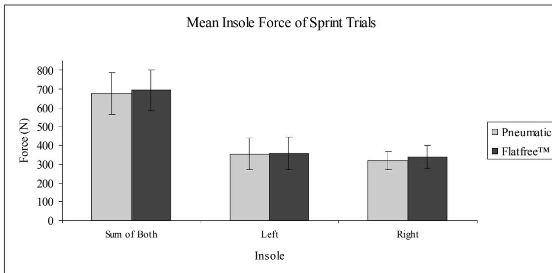
Figure 3. The total mean ( $\pm$ SE) of force for both insoles (left + right), the left insole and the right insole for the pneumatic and Flatfree™ trials for the 10 second sprint trials.
