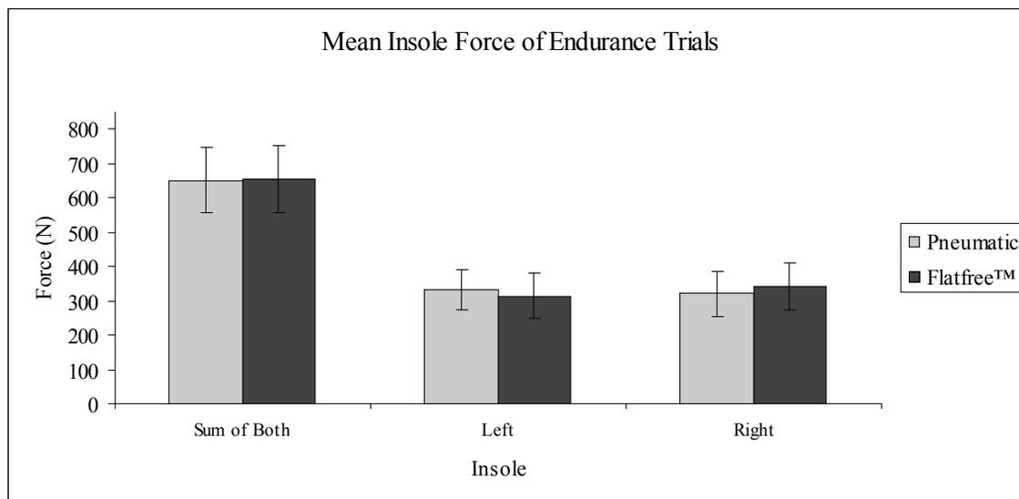
Figure 4. The total mean ( $\pm$ SE) of force for both insoles (left + right), the left insole and the right insole for the pneumatic and Flatfree™ trials for the 20 minute endurance trials.
