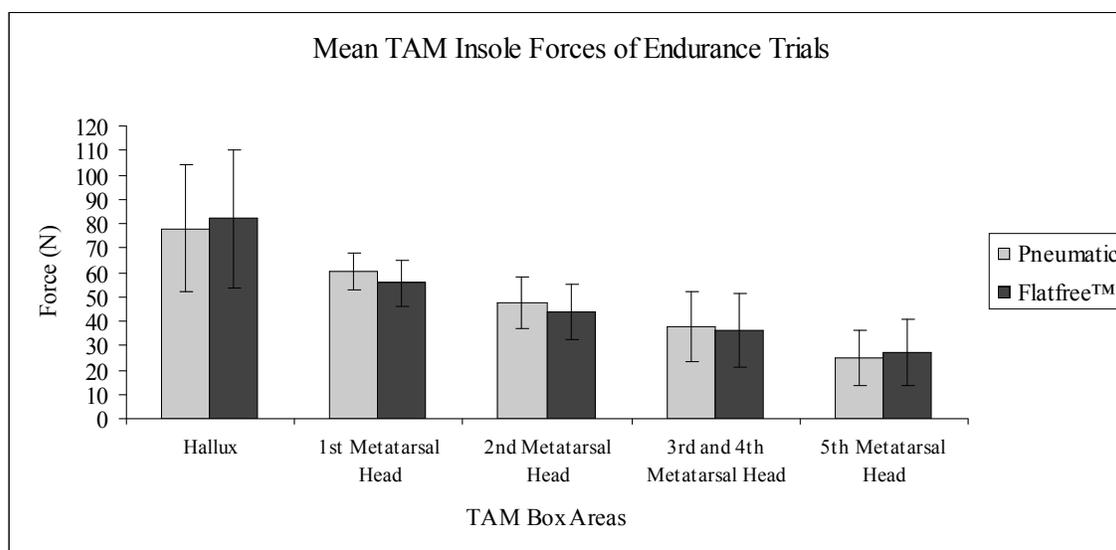
Figure 6. The mean forces ( $\pm$ SE) of both insoles utilizing the TAM box areas of the F-scan® program are displayed for the pneumatic and Flatfree™ tires during the 20 minute endurance trials.
