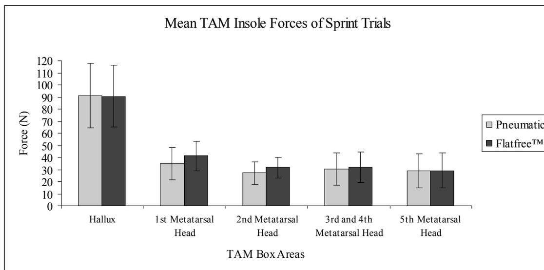
Figure 5. The mean forces ( $\pm$ SE) of both insoles utilizing the TAM box areas of the F-scan® program are displayed for the pneumatic and Flatfree™ tires during the 10 second sprint trials.
