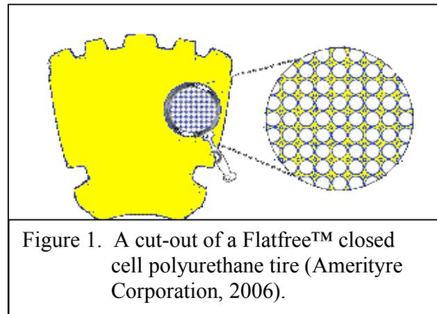
wear fairly well. Their higher spring constant than pneumatic tire has the tendency to generate a rougher ride than pneumatic tires. It has been observed that these closed cell tires are manufactured in a variety of fashions in the automotive industry such as a liquid injection molded tire or cast tire that is similar in form to a traditional pneumatic (Morgan, J., 1981). These have a low rolling resistance but also a higher spring constant
